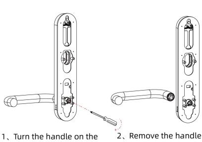
1. Turn the handle on the front panel Loosen the inner hexagon screw of the handle counterclockwise
