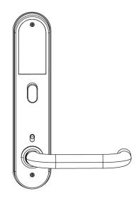
3. After adjusting the direction of the handle, insert it into the handle seat and re-lock the hexagon screw of the handle to the complete the turning
